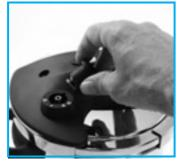
The valve can now be lifted off and removed upward from its catch. Clean by running under water and reinsert into catch.
